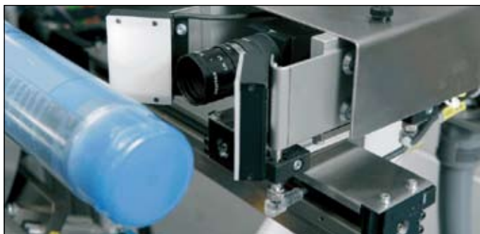
An array camera determines the exact radial and axial position using the tube's print image
