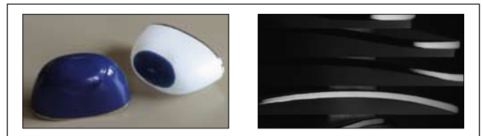
Oval Cap with hot foil print, image sequence of half a revolution, the second half is symmetric
